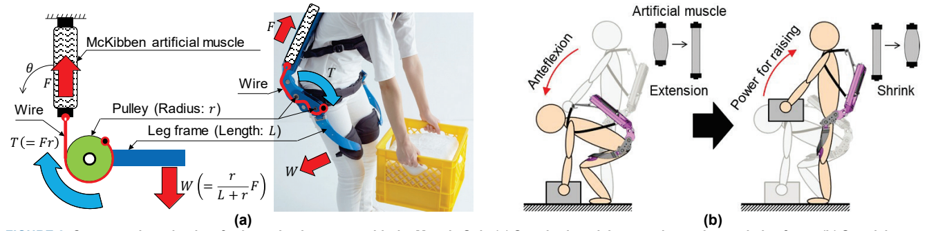
FIGURE 2. Conceptual mechanism for lower back support with the Muscle Suit. (a) Standard model generating active assistive force. (b) Standalone model generating passive assistive force.
